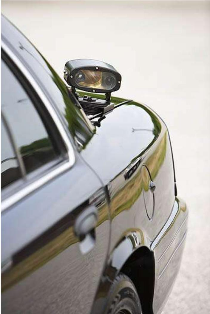
The core of the system is the AD3 split camera. This is a pair of intelligent digital cameras (one B&W with infrared illuminator and one colour) housed in a compact, ruggedised, nitrogen-filled casing. The cameras can be mounted on magnetic bases or on roof bars. Cameras are provided in 16, 25 and 50 mm focal lengths that provide a blend of close-up reads (e.g., for cars parked on the left side of a road) and oncoming traffic across multiple lane reads.
