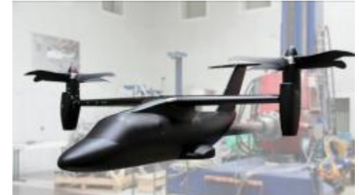
1:5 Powered model wind tunnel test
