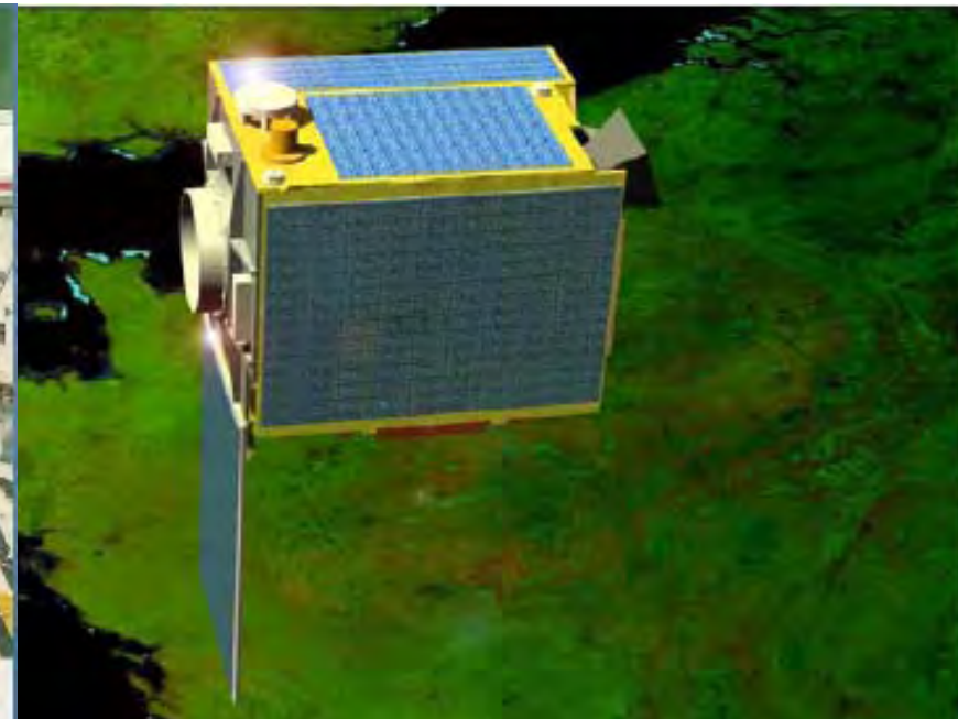
Proba-V Dimensions 800mm x 800mm x 1000m
